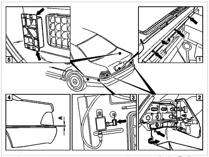
Expanding rivet (Fig. 1) remove.
